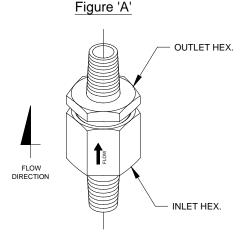
Products that utilize SAE J1926/2 (S-Series) threads or BSPP ISO-228/1 (BS 5380) threads require the use of an O-ring to seal. O-ring to be provided by the customer.
