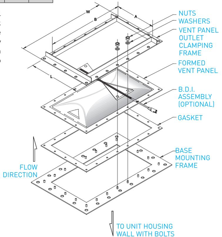
**TABLE 3 // CFR and CFS Vent Panel Frames**
